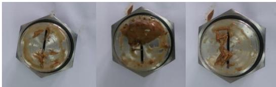
Figure 1. No bridging material formed in the fractures
