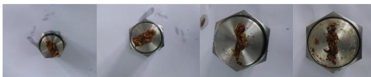
Figure 2. Bridging material formed in the fractures
